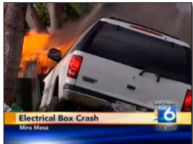
Figure 22-19 Vehicles can become energized when contacting Live Front Terminator Boxes
