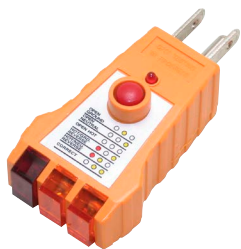
Figure 22-21 Slater Circuit Tester used to check correct wiring of an outlet
