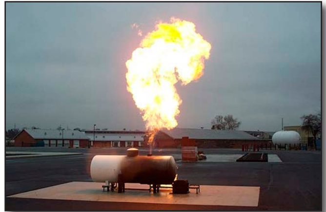
Figure 22-36 Venting LPG Tank
